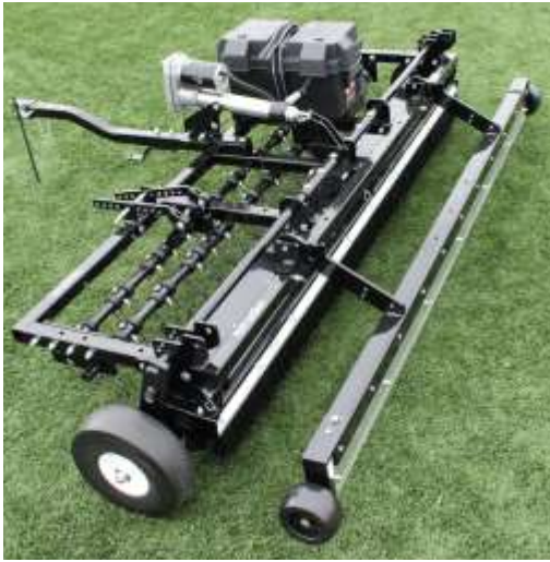
Turf Setup. Broom Carriage with optional Rear Magnet.
