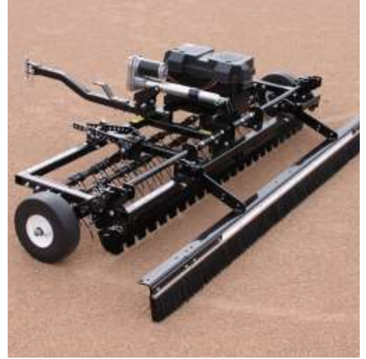
Infield Setup. Leveling Implement with Rear Smoothing Broom.
